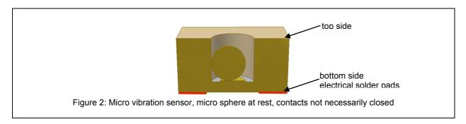
The unidirectional sensor version MVS1006.01 is open at rest, when mounted in upside down position, so that the micro sphere is on the top side of the sensor, which has no contact pad.
